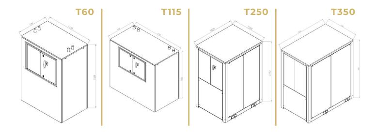
NOTE: For **T60** and **T115** the following clearances apply: front and rear 500 mm, side left and right 600 mm and top 500 mm. For **T250**, **T350** the following clearances apply: front and rear 1000 mm, side left and right 800 mm and top 150 mm.
