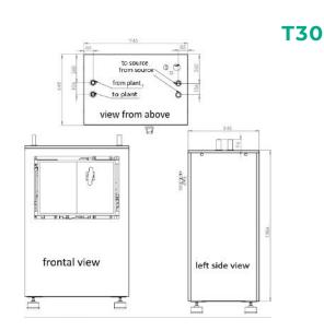
$NOTE: For both ~\textbf{710} \ and ~\textbf{730}, the following clearances apply: front and rear 500 \ mm, side left and right 600 \ mm and top 500 \ mm.$
