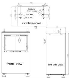
NOTE: For both **T10** and **T30**, the following cle es apply: front and rear 500 mm, side left and right 600 mm and top 500 mm.
