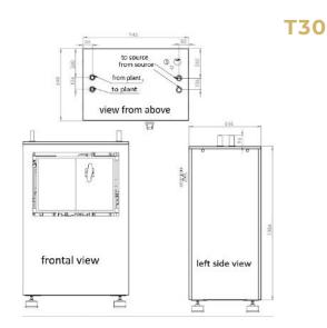
NOTE: For both T10 and T30, the following clearances apply: front and rear 500 mm, side left and right 600 mm and top 500 mm.
